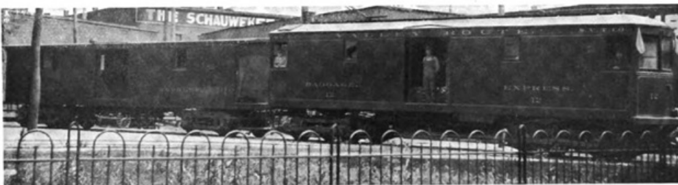
MOTOR AND TRAILER FOR EXPRESS AND FREIGHT SERVICE, SCIOTO VALLEY TRACTION
